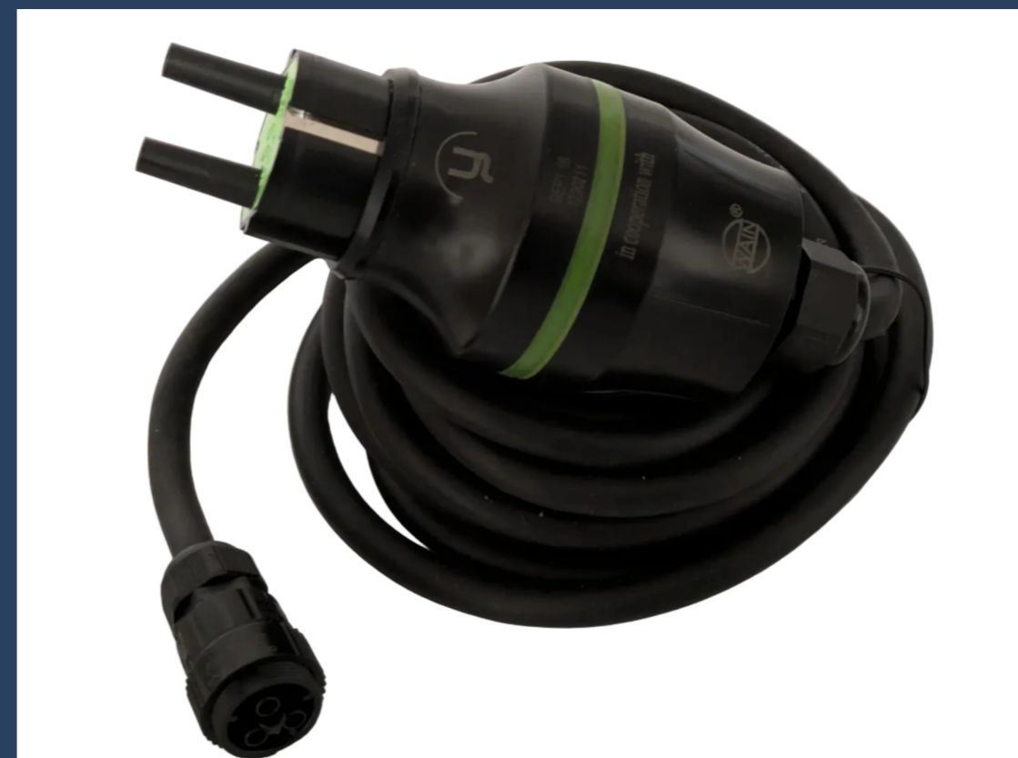
Seplugins adds retracting sleeves over the pins to a standard European plug to provide touch protection without requiring a special socket. Photo: Seplugins.
